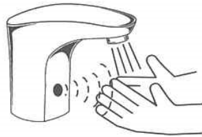
Put hand in front of the sensor window, Sensor detects and water come out automatically
